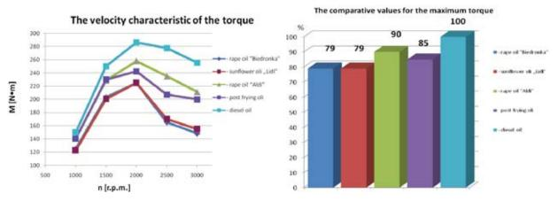
Fig. 2. The velocity characteristic of the torque and the comparative values for the maximum torque
