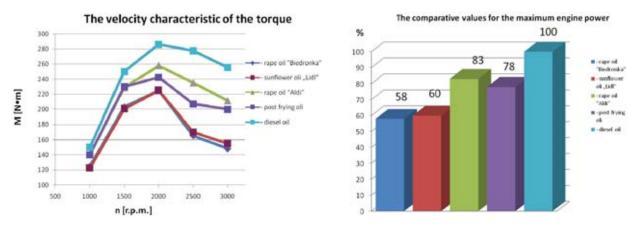
Fig. 3. The velocity characteristic of the engine Power and the comparative values for the maximum engine power
