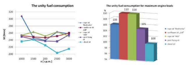
Fig. 4. The unity fuel consumption for the full characteristic and for maximum engine loads
