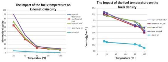
Fig. 1. The impact of the fuels temperature on kinematic viscosity and on the fuels density
